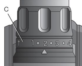
fastener at the desired depth. The lower the number, the lower the torque output.
