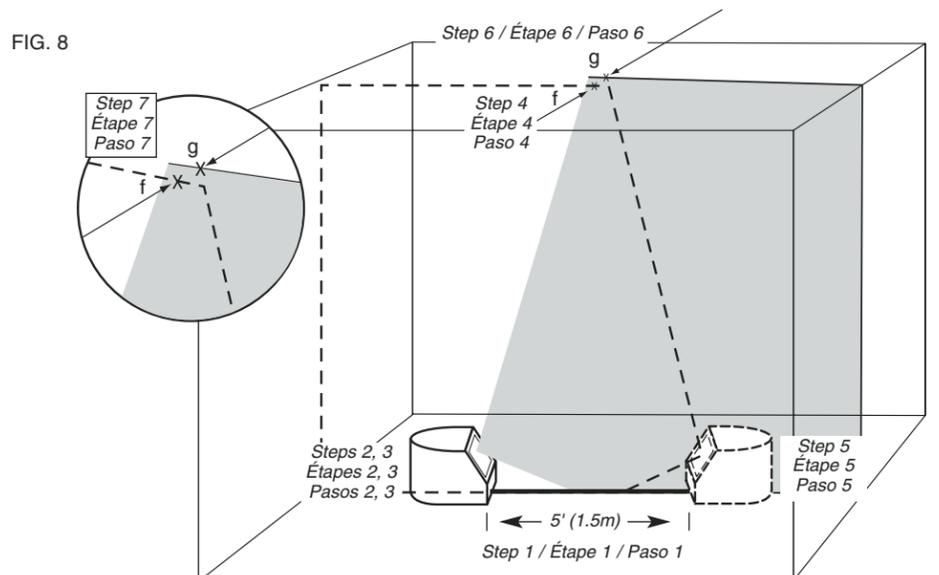
5. Reposition the laser at the other end of the line on the floor. Adjust the unit once again so its beam is aligned and centered on the line on the floor.
